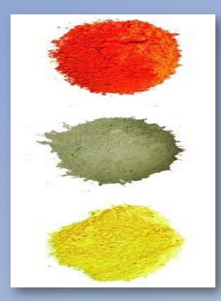
LEAD PRODUCTION (LITHARGE, REFINED LEAD, RED LEAD & GREY LEAD)
