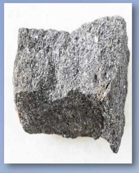
Chromite is an oxide of chromium and iron. The chemical composition of chromite is FeO.Cr2O3 or FeCr2O4. Chromite is the only commercial source of chromium. It occurs as a primary mineral of ultrabasic igneous rocks and is normally associated with peridotite, pyroxenite, dunite and serpentinite.....Read more
